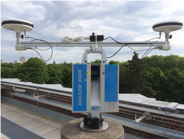
TLS-Based MSS For Directly Geo-Referencing ( dirGref 2015) 3D Point Clouds
