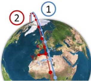
Two ascending Collinear Tracks along which GOCE gradients are compared
