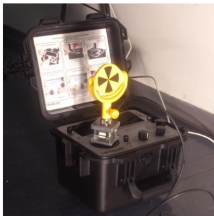
ATTACHED PASSIVE TARGETS TO THE PORTABLE SHAKER VIBRATION CALIBRATOR 9210D (LEFT) AND ESTIMATED FREQUENCY OF 1 HZ AT SLOPE DISTANCE OF 5 METER (RIGHT)
