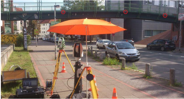
VIBRATION ANALYSIS OF THE FOOTBRIDGE STRUCTURE USING THE TELESCOPE CAMERA OF THE MS50 TO MEASURE A PASSIVE TARGET ATTACHED TO THE SIDE OF THE FOOTBRIDGE .
