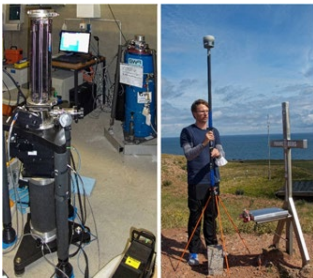
(LEFT) SIMULTANEOUS MEASUREMENTS WITH THE HANNOVER ABSOLUTE GRAVIMETER AND THE SUPERCONDUCTING GRAVIMETER OF GFZ POTSDAM; (RIGHT) MEASURING HELGOLAND'S COASTLINE, LAND TOPOGRAPHY AND TIDE GAUGES WITH REGARD TO THE GRAVIMETRIC SENSORS ON THE UPPER LAND AND IN THE HARBOUR (HERE WITH DR. CHR. VOIGT, GFZ POTSDAM).
