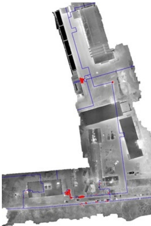
ANOMALY DETECTION: THE POSITIONS OF THE PIPES ARE MARKED WITH BLUE LINES AND THE ANOMALIES ARE SHOWN BY RED
