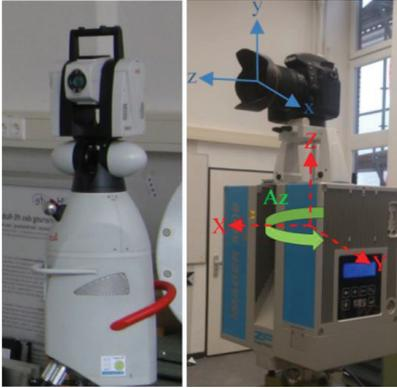
**LEICA AT901LR LT (LEFT), A NIKON D750 24.3-MEGAPIXEL DIGITAL CAMERA IS RIGIDLY MOUNTED ON TOP OF THE Z+F IMAGER 5006 TLS (RIGHT)**
