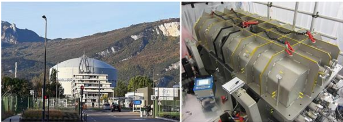
LEFT: AT ILL GRENoble, GRAVIMETRIC MEASUREMENTS WERE PERFORMED IN THE BUILDING WHICH IS ACTUALLY A NUCLEAR REACTOR WITH A POWER OF 58 MW, NEEDED AS THE NEUTRON SOURCE FOR THIS PHYSICAL EXPERIMENT. RIGHT: THE HANNOVER RELATIVE GRAVIMETER SCINTREX CG-6#171 IS MEASURING CLOSE TO THE SITE WHERE THE NEUTRONS ARE INTERROGATED FOR THEIR ENERGY LEVEL (PHOTO LEFT: L. TIMMEN, RIGHT: H. DENKER)
