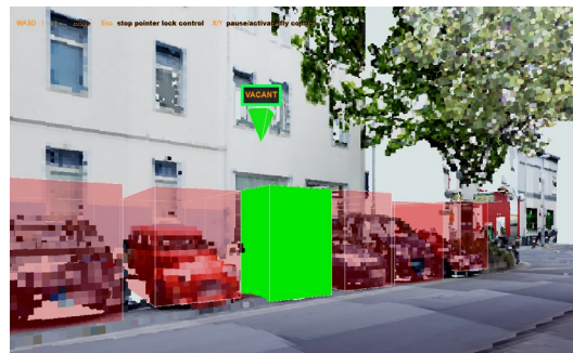
ABBILDUNG 2: THE URBAN DIGITAL TWIN VISUALIZATION WITH COLORS DERIVED FROM CAMERAS, WITH INTERACTION POSSIBILITIES FOR PARKING SPACE MANAGEMENT USE CASE. THE GREEN BOX INDICATES THE VACANT PARKING SPACE, WHILE THE RED BOXES REPRESENT THE OCCUPIED PARKING SPACES.
