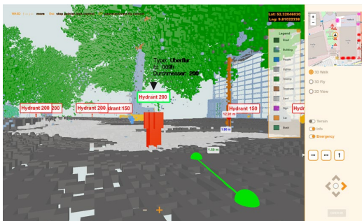
ABBILDUNG 1: THE WEB APPLICATION OVERVIEW WITH DIFFERENT INTERACTION POSSIBILITIES FOR SPECIAL OPERATIONS FORCES (FIREFIGHTERS) USE CASE. THE URBAN DIGITAL TWIN IS REPRESENTED WITH SIMULATED COLORS ACCORDING TO THE CLASSIFIED DATA
